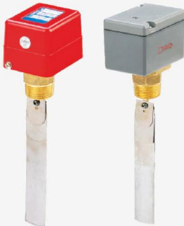
Series liquid flow switch is designed for managing the flow changes when the liquid flows in the pipe, such as water, ethylene glycol or other non hazardous liquids. When the liquid flow is higher or lower than the setting value, the single pole double throw contacts (SPDT) can get through one circuit and at meantime to break the other circuit. Series liquid flow switch is commonly used for chain reaction or "no flow" protection.
