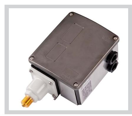
The RT-E series consist of pressure and differential pressure switches as well as temperature switches. The units are designated for industrial refrigeration and general industrial application in explosive zones acc. to 94/9/EC, Atex directive, explosive zone 1, for surface equipment, category 2.
