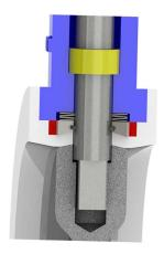
Disc spring,two sets for a group,is a state of compressive deformation in the body. It will impose elastic force on the press sleeve,compact the O ring and seat,improve axial sealing,then provided the bearing stress for the seat and disc,to cover the shortage of elasticity about PTFE seat.
